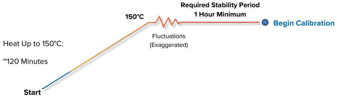
Figure 3: Oven Chamber Heat Up and Stabilization Phases
