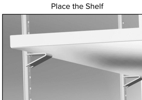
1. Install the shelf clips in the slots of the shelf standard mounting rails located on the sides of the chamber interior, 4 clips per shelf.
