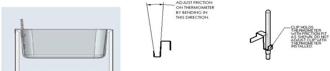
**Note:** Water bath thermometer must be placed so that the bulb is always fully immersed. The thermometer must not touch the sides or the bottom of the bath tank.
