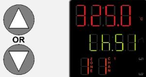
Use the [Set the High Temperature Limit](#) procedure on page 27 to set the Limit heating cutoff to at least 10°C above the highest intended temperature of your application.
