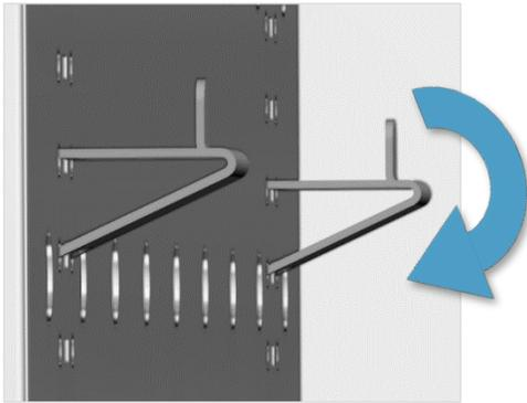
**Figure 5: Install Clips**
