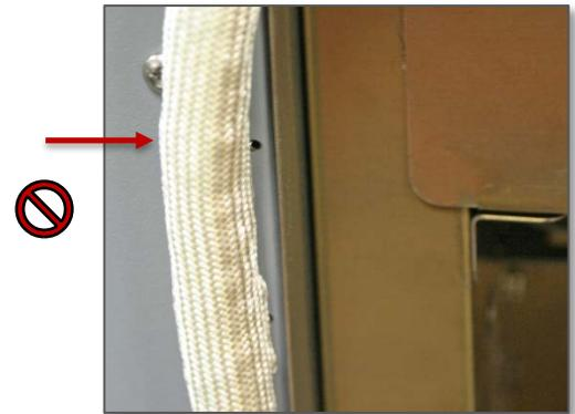
**Figure 8: Chamber Gasket Misaligned**
