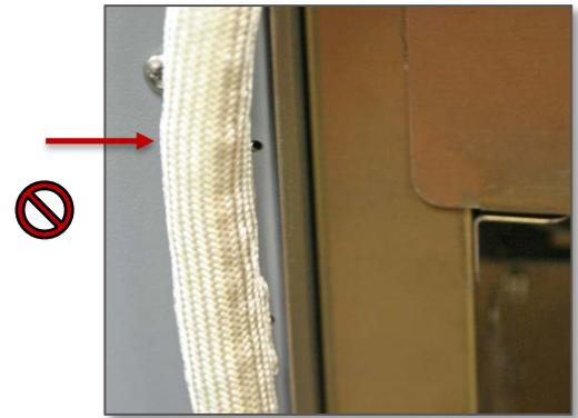
**Figure 8: Chamber Gasket Misaligned**
