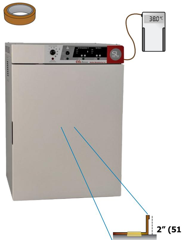
**CO<sub>2</sub> Calibration:** A CO<sub>2</sub> calibration may be performed during the temperature calibration so long as the chamber door and access port remain closed and sealed.
