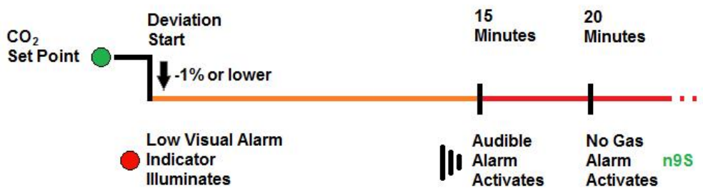
Low and No Gas Alarms Timeline
