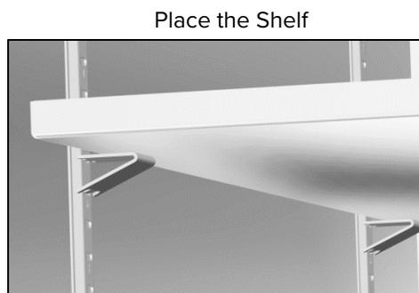
1. Install the 4 shelf clips in the slots of the shelf standard mounting rails located on the sides of the chamber interior.
