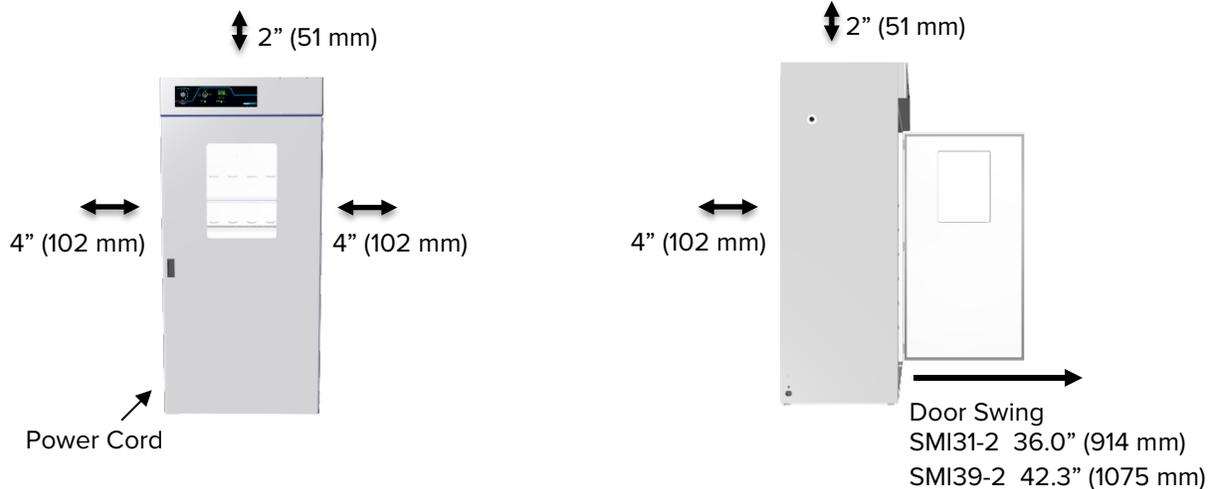
**4 inches (102 mm)** of clearance is required on the sides and back.
