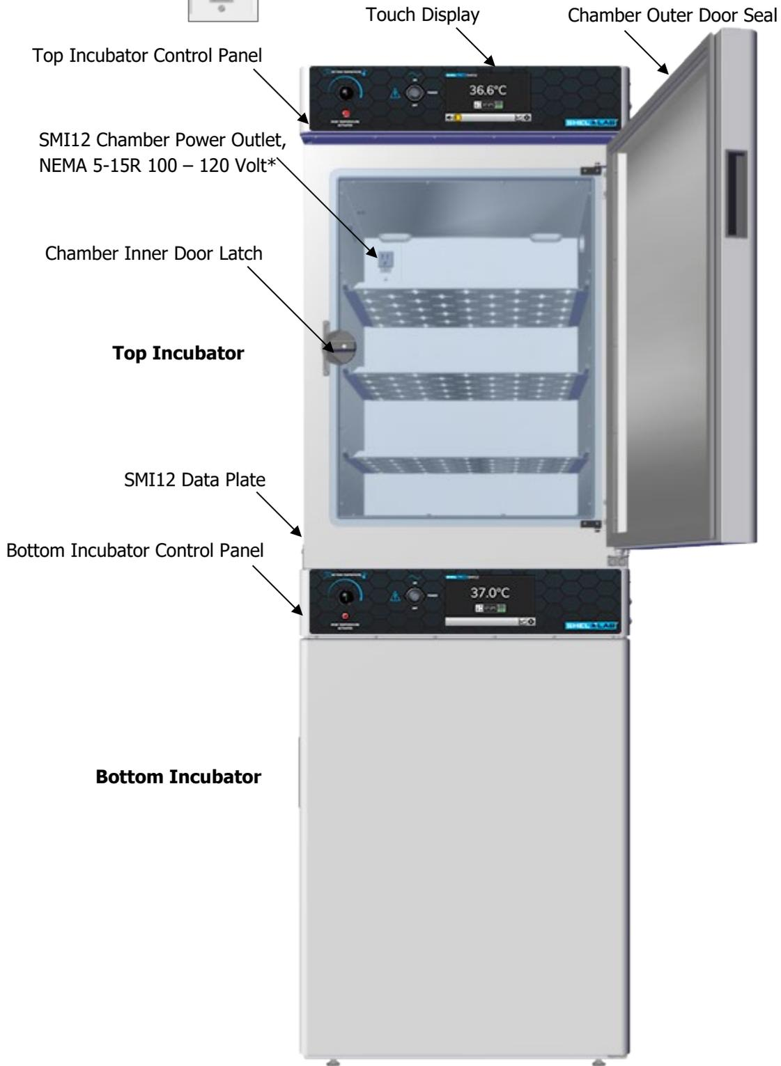
**Note:** The SMI12 consists of two SMI6 incubators secured to a stacking brace. Each incubator operates independently and is separately powered.
