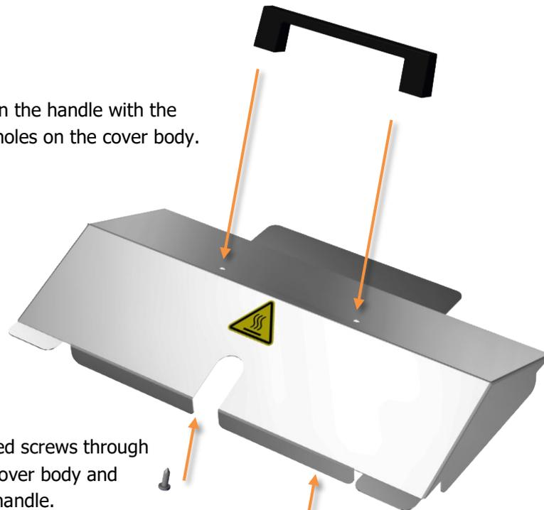
**2.** Insert the 2 included screws through the underside of the cover body and into the holes on the handle.
