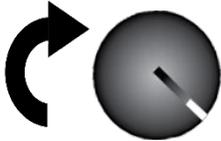
Turning the OTL to the far right (clockwise) prevents the heating cutoff system from interfering with this procedure.
