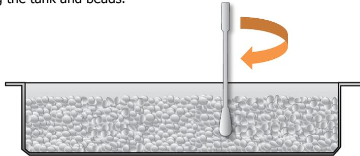
2. Load samples in the tank. Ensure that the combined volume of samples and beads does not cause the tank to overflow.
