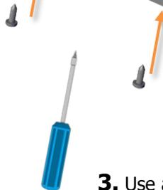
**3.** Use a **Phillips screwdriver** to tighten the screws until the handle is securely fastened. Do not overtighten.
